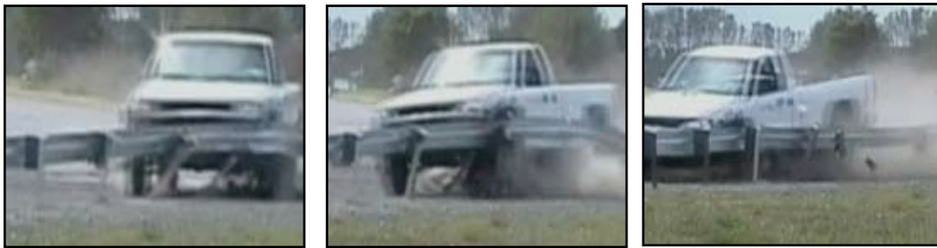
Test Level 3 crash test of NU-GUARD-27 design.
